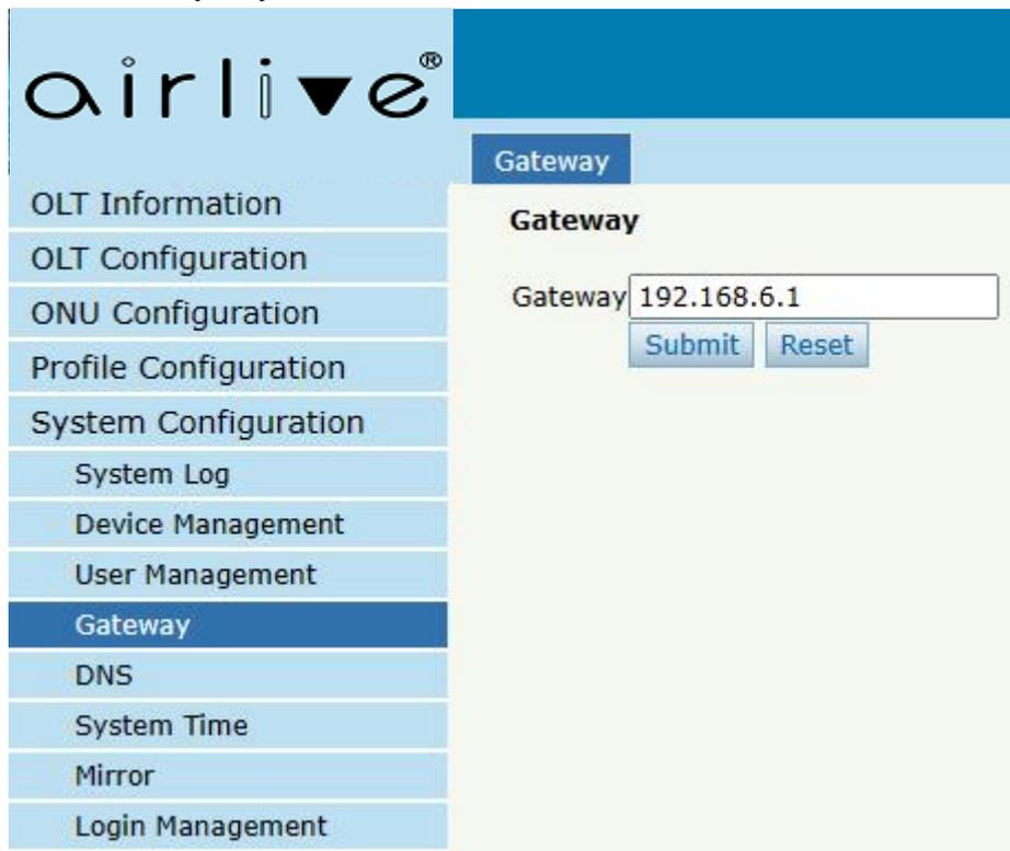
Figure 6-5-1: Gateway Configuration
